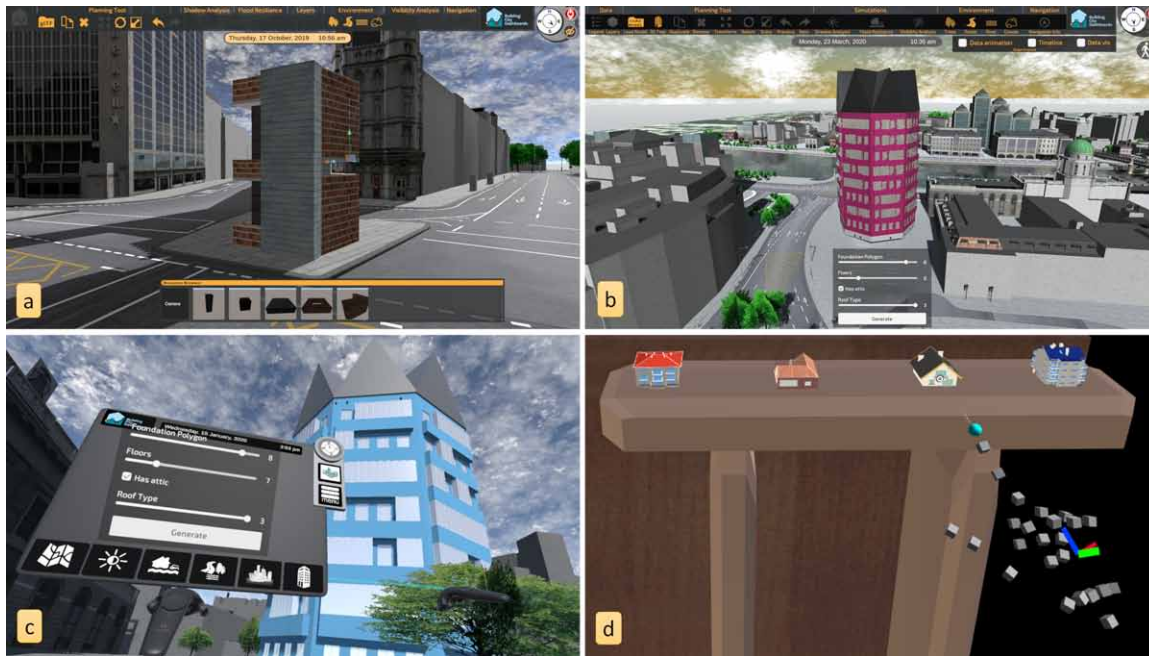
Figure 9. Runtime 3D modeling tool, interactive buildings library: (a+b) desktop; (c) VR; (d) MR
