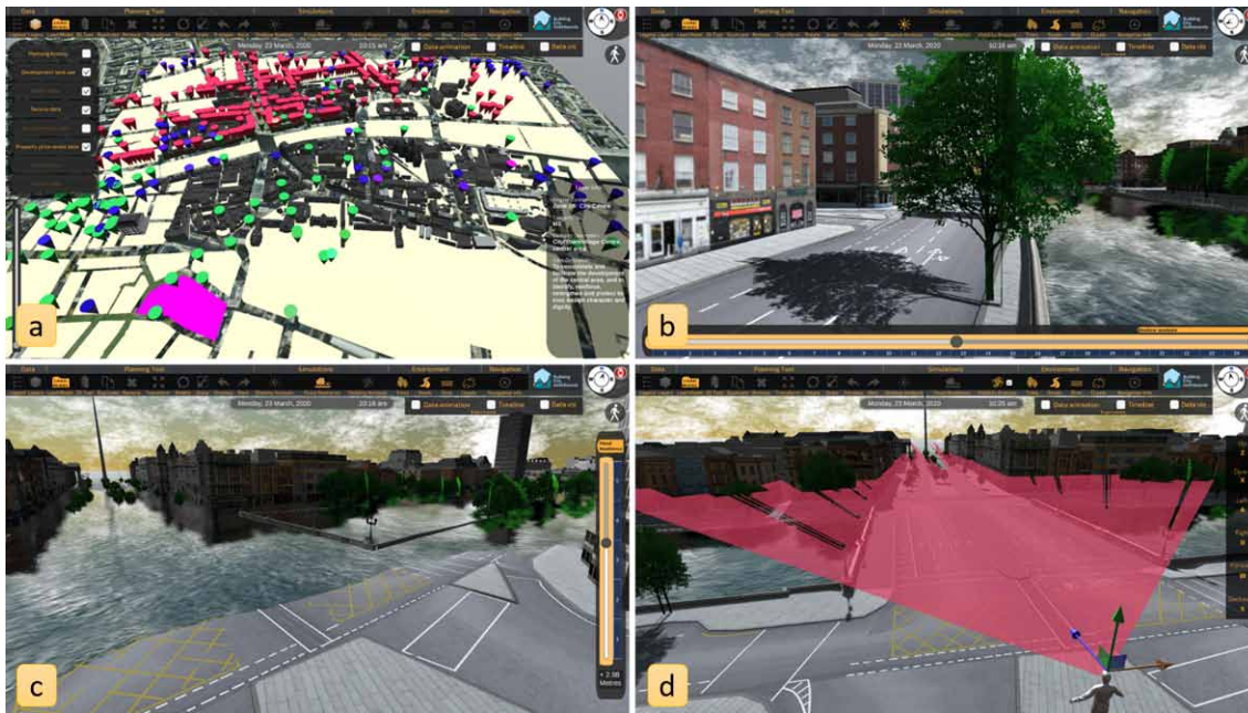
Figure 7. BCD desktop app: (a) interactive city layers; (b) shadow analysis; (c) flood resilience; (d) visibility analysis
